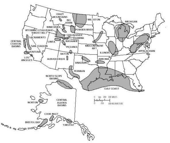
Figure 1. Map of the United States showing basins containing sedimentary rocks more than 15,000 ft. (4,572 m) deep. Shading indicates entire basin area, in which some of the sedimentary rocks are at shallow depths.<sup>13</sup>
